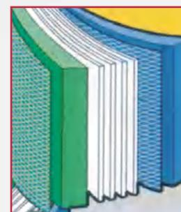
**Ultra-high-efficiency degreasing filters:** corrosion-resistant inner/outer cartridges, external coated closed-cell foam sleeves
